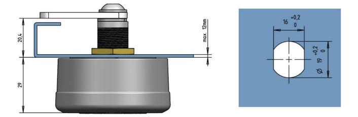
2. Fastening in wooden doors by means of cup drilling and optional anti-rotation bolt (Specify when ordering)
