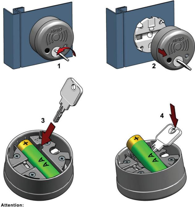
Make sure the polarity is correct when inserting the battery! Batteries inserted the wrong way round can damage the electronics or destroy them.
