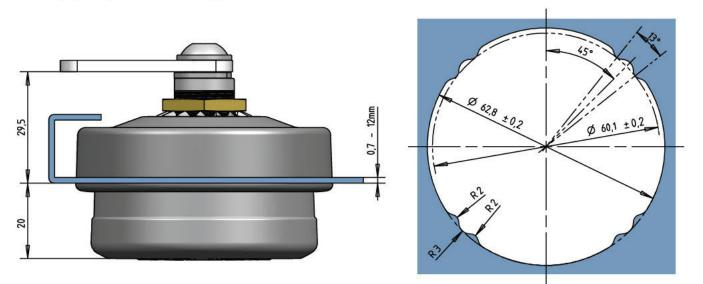
2. Recessed installation in wooden doors using special milling and optional installation shell (Specify when ordering)
