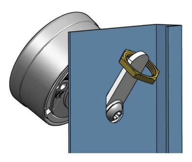
2. Assembly sequence for separately delivered cams
