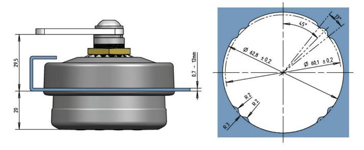
2. Recessed installation in wooden doors using special milling and optional built in shell (Specify when ordering)
